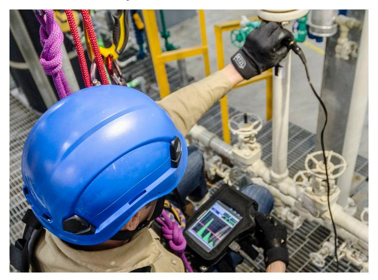
The workflow of the EPOCH® 6LT flaw detector is simple and straightforward. The primary screen is a large, optimized A-scan display that contains links to commonly used features and functions. Combined with an improved scanning workflow, users can complete their inspections with minimal button presses and adjustments. When you do need to navigate the menu, prominent icons make it easy to find the feature you're looking for.
